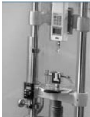
Fig. 5: SH-500 pull and push dynamometer
