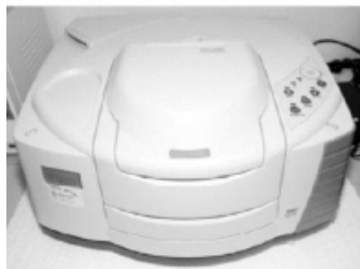
Fig. 6: Fourier transform infrared spectroscopy (FTIR)
